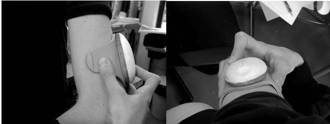
Figure 5. Prototypes exploring the monitor's attachment to the wings and the wings' attachment to the arm.
